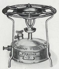
Strongly constructed of Heavy Gauge Brass, Copper Plated Burner, Stamped Steel Top Plate. Capacity of Tank  $2\frac{1}{8}$ -pints. Silent Burner for indoor burning. Roarer Burner for out-of-door
