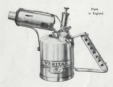
Veritas Mark I Blowlamps are made in first quality Heavy Gauge Brass, with indestructible perforated steel handles which always remain cool. The 1-pint size generates an intensely hot flame of approximately 3,000 deg. Fahr. They are unaffected by rain and wind and will burn in practically any position. Indispensable for plumbing, burning off paint, soft soldering and light brazing operations.
