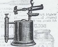
Heavy Gauge Seamless Brass, Reinforced Tank with Concave Bottom and Filler Plug, with Lead Gasket; Automatic Pump in Handle; Single Piece Straight Tube Burner gives intense blue flame; With Hook and Support for Soldering Coppers; For home use, paint burning, thawing pipes and light repair work.
