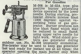
operator opening the main burner only when desiring the powerful blast flame.
