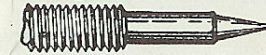
Sharp Pointed Needle Quickly ruins the Burner by forcing Orifice larger if the operator does not take proper care.
