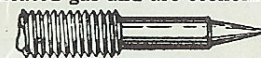
Sharp Pointed Needle Quickly ruins the Burner by forcing Orifice larger if the operator does not take proper care.
